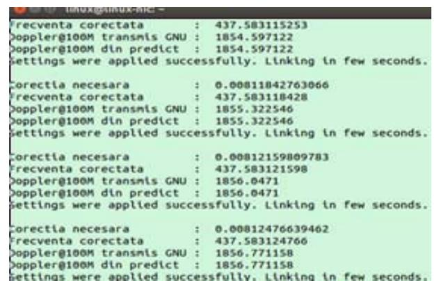
Figure 7. Doppler correction send to GNU Radio.
