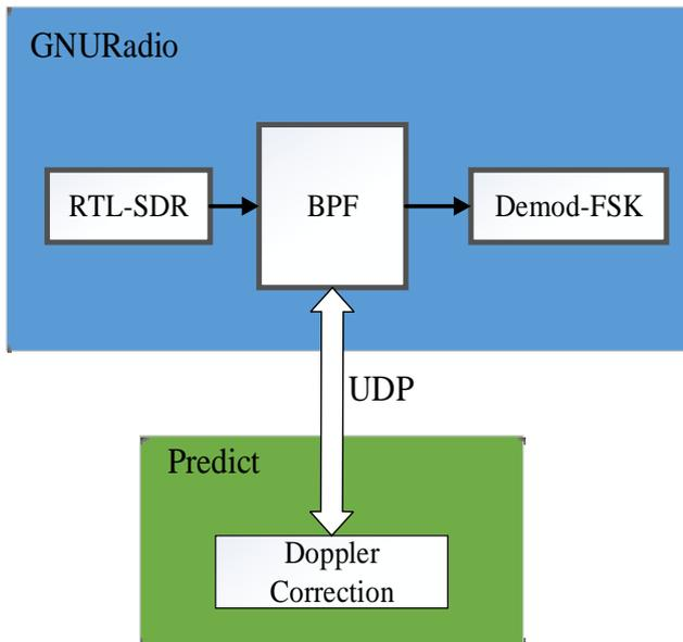
Figure 4. Doppler correction diagram.
