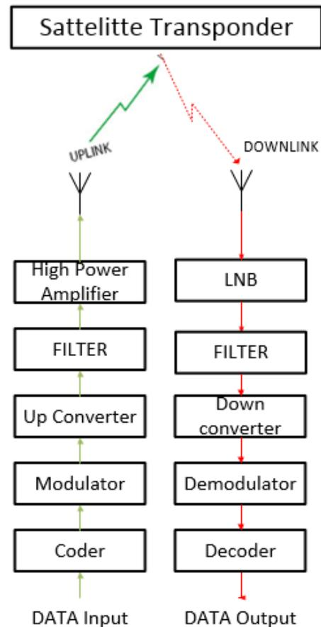
**Figure 1.** Traditional radio architecture.
