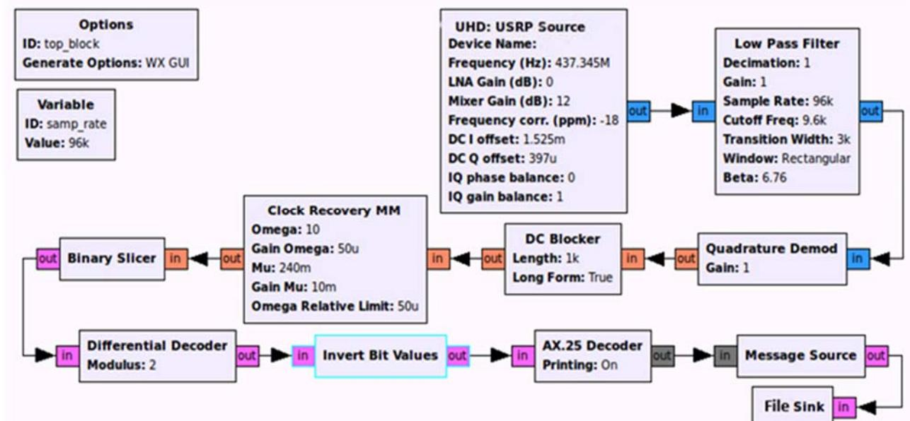
Figure 9. Implementation of created digital signal processing block
