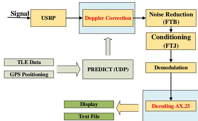
Figure 3. The reception of telemetry information in GNU Radio.
