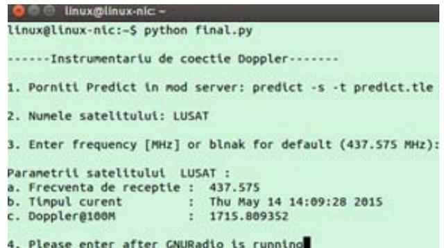
Figure 6. Developed script for Doppler acquisition.
