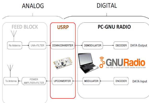
Figure 2. Software Defined Radio Architecture.
