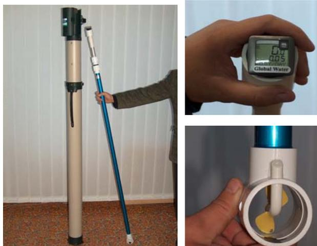
Figure 2 - FP 201 Global Water Flow Probe.
